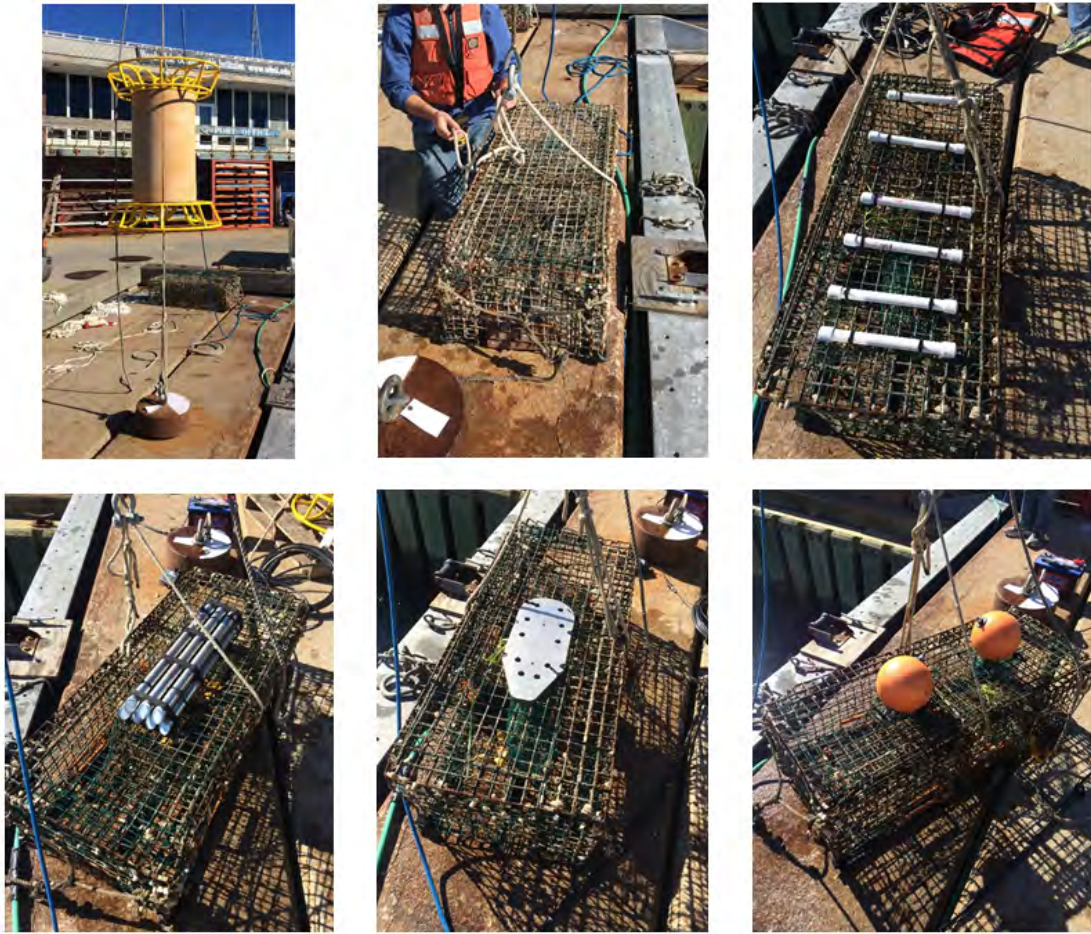
Figure 6.2: Different experimental treatments measured. From left to right, top: Line pack spool and anchor; bare lobster trap (22" x 48" x 14", previously fished in Cape Cod Bay); lobster trap with six \frac{3}{4} " x 12" PVC pipe reflectors. Bottom: lobster trap with seven grouped 1.5" x 24" metal tube reflectors; lobster trap with 7" x 20" x \frac{1}{2} " steel plate; lobster trap with two 7" trawl floats.
