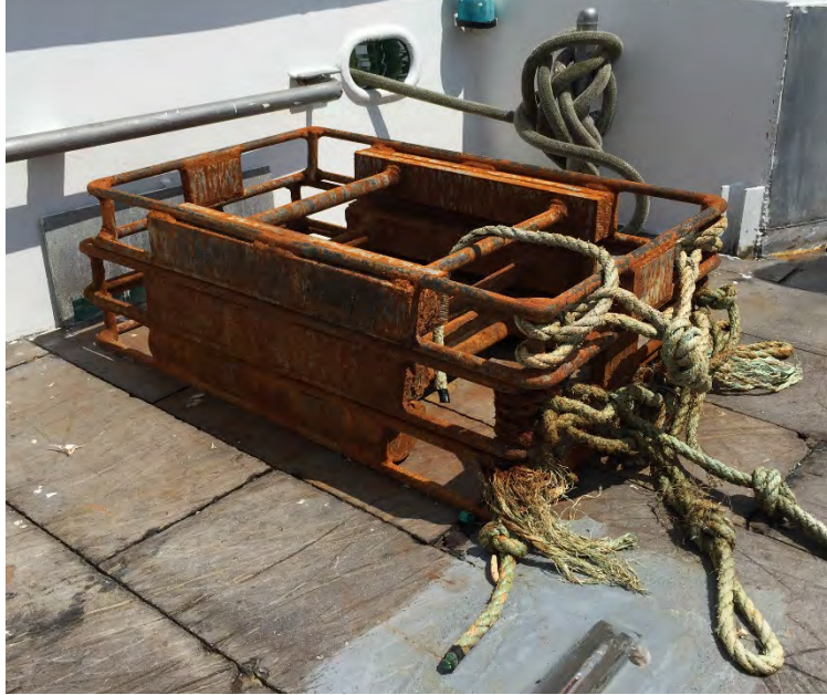
Figure 1.2: Two 180-pound steel anchor sleds. The anchor sleds weigh more than the empty line pack spool (about 135 pounds), i.e. the line pack spool weight is comparable to weights of existing gear.
