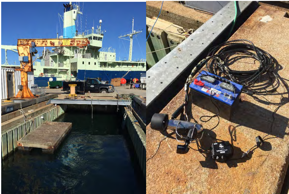
Figure 6.1 Left: The well at the WHOI dock where the experiments were performed. It is approximately 45-50 feet deep, with a crane and an opening that is 18 feet wide. Right: The Vexilar SonarPhone used for the sonar imaging, showing the "towfish" weight that was used to depress the sonar transducer and tow it back and forth across the well.
