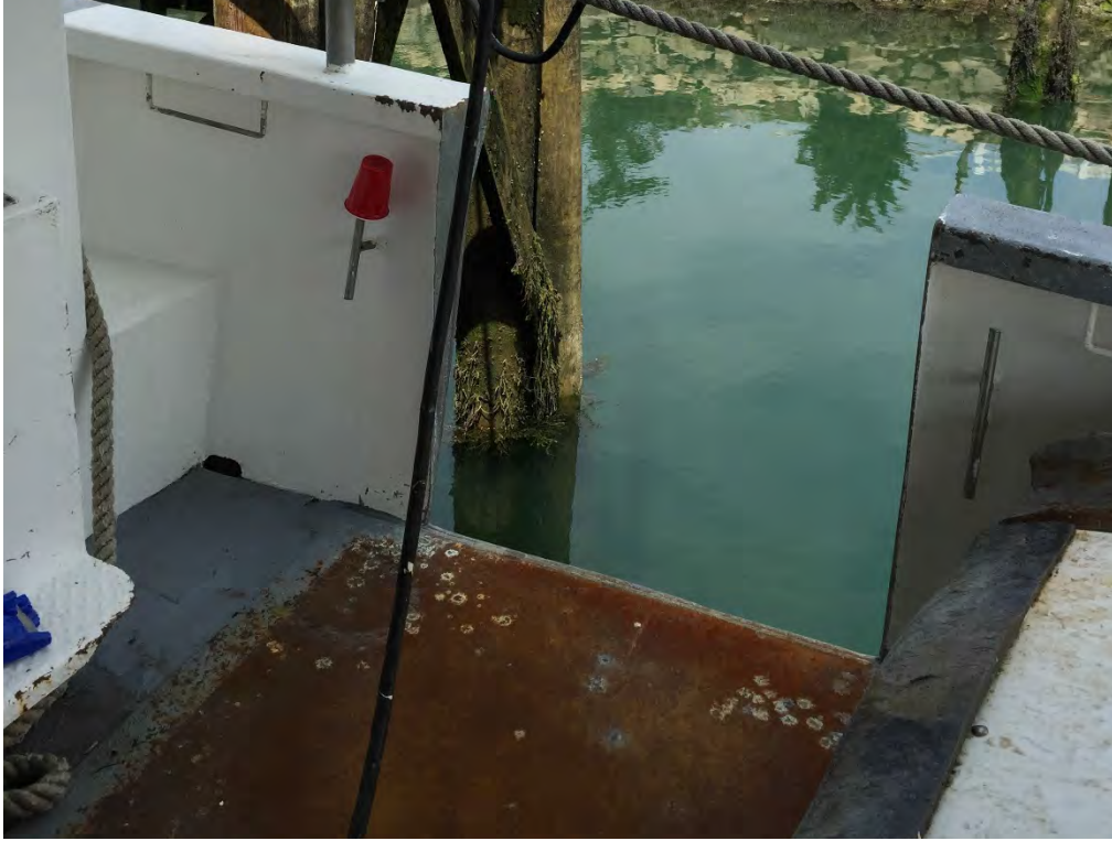
Figure 1.4: Opening in rail through which gear is hauled. The line pack spool is 32" wide and 43" tall.
