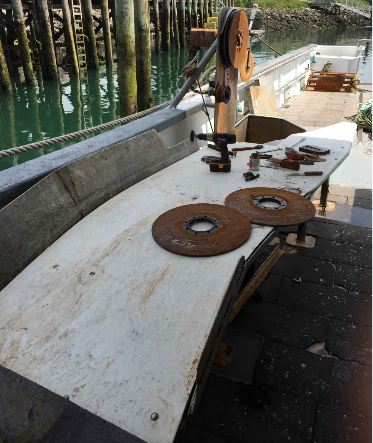
Figure 1.6: Pot hauler, pot hauler plates, rope locker, anchor sleds, line.
