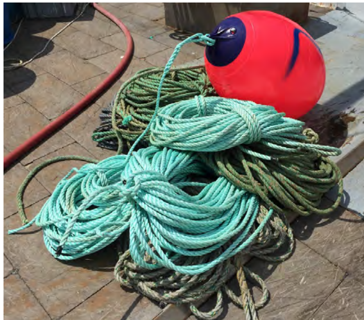
Figure 1.1: 300 fathoms (600 meters) of 5/8" line, coiled in 50-fathom shots, with one Polyform LD-3 float. This is the typical amount and diameter of line used for one of the vertical lines in an offshore trawl in 100 fathoms of water with high surface currents. Often two Polyform LD-3 floats will be used for increased floatation.
