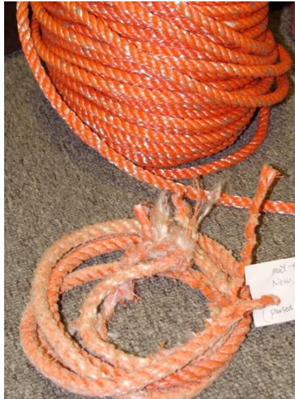
Figure 5. A portion of sinking groundline that parted after only three hauls, compared to new rope behind it. (Photo L. Ludwig)
