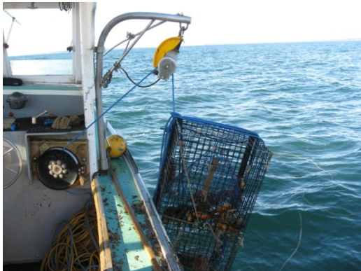
Figure 8. Lobster trap wrapped in sinking line. (Photo J. Alley)
