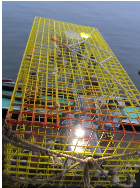
Figure 13. The experimental trap with three cameras mounted inside and additional lighting.
