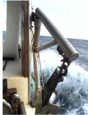
Figure 7. Bent davit. (Photo C. Moore)
