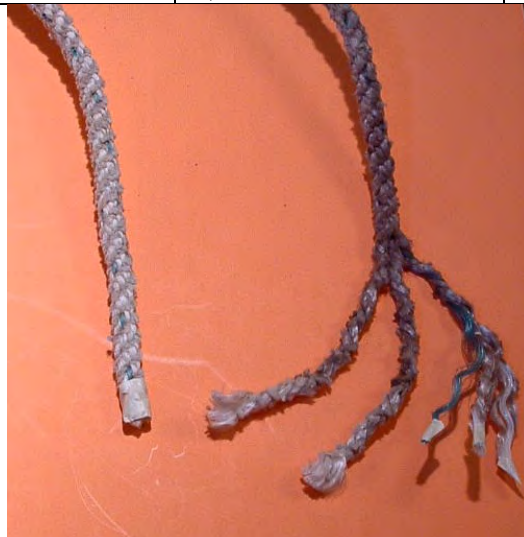
J031704 \frac{3}{8} 3-Strand PP/PET blend. Note uniform surface abrasion.
