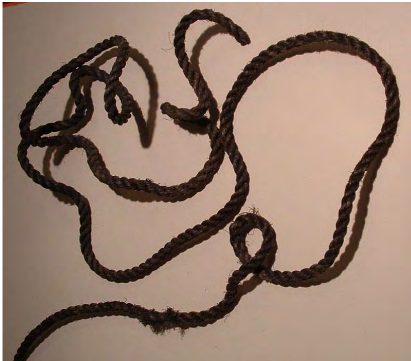
J071795-a Note kinks and cut at bottom of photo.
