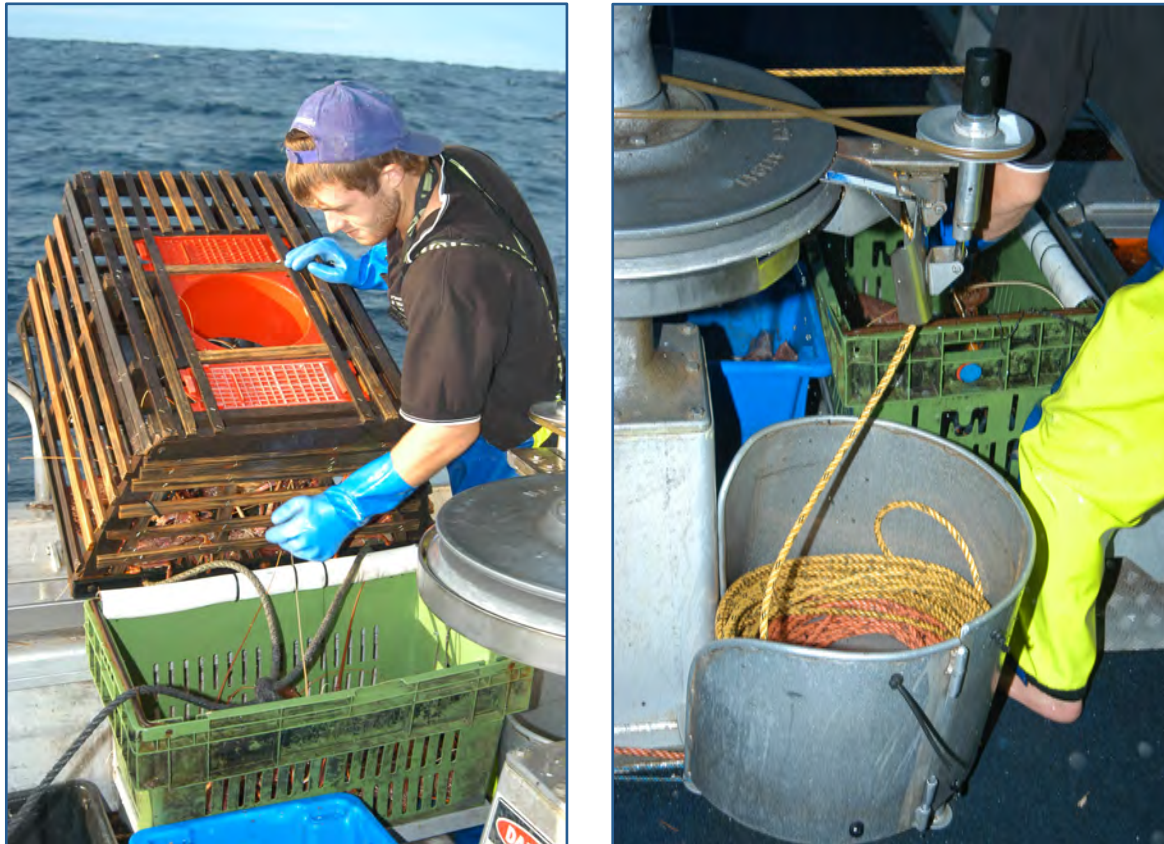
Figure 4. Emptying a wooden, top entry lobster pot (left), and the rope hauling/coiling mechanism.
