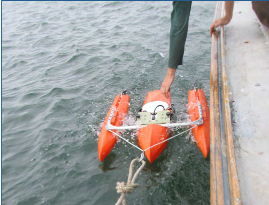
Figure 2. ADCP with catamaran deployed next to a lobster boat.
