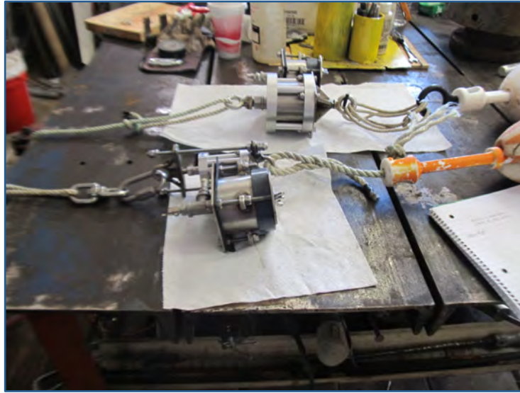
Figure 1. Two self-recording load cells designed and built by Blue Water Concepts.
