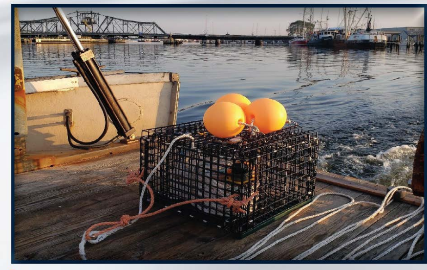
Figure 7. The Edgetech trap in which the vertical line is contained at the seafloor.
