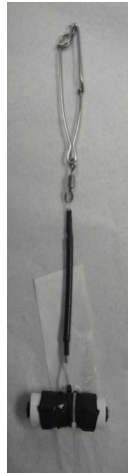
Figure 7. Completed capsule with neoprene sleeve, attachment clip, and leader
