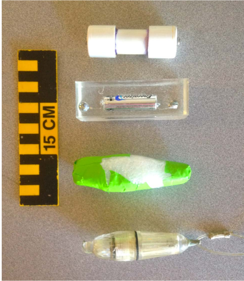
Figure 4. Side-by-side comparison of modified “version two” design for a device to attract pelagic elasmobranchs away from the baited hook on pelagic longline gear. This version is potted within solid clear acrylic to avoid leakage problems with “version 1.0” device (top), and includes a AA-size battery, a resistor, and two screws (grey arrows on diagram below) exiting the acrylic to create the electric field. The “version 2.0” is the rectangular clear block (top middle), with the screws (contact points) exiting on one side of the device. The newest “version 2.1” is similar in size in shape to the clear, cylindrical object (bottom), although constructed of clear acrylic and with contact points on either end. The “version 2.1” dummy block for the mold is included (bottom middle) to provide a sense of scale of this version of the device. The actual device is not shown.
