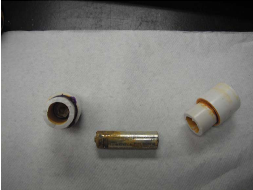
Figure 9. Failed capsule cut open, showing water leak damage.
