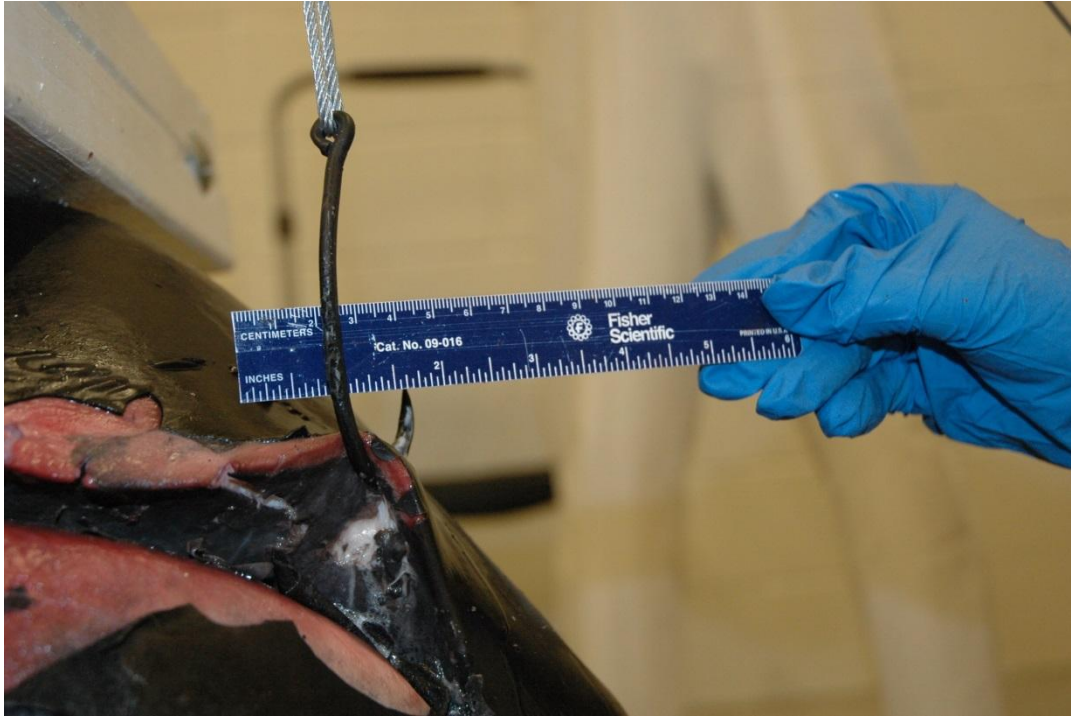
Figure 24. View of the tissue of dorsal caudal lip of a short-finned pilot whale with a Korean Carbon 16 hook being pulled to 156 kg of force. The soft tissues resist tearing even under this high load.
